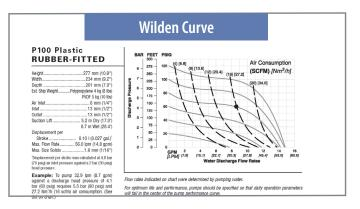
The manufacturers of pirated parts will oftentimes create a "cut and paste" reproduction of the part's performance information that comes straight from the manual of the original manufacturer. In this example, there is no real discernible difference between the flow curve for JDA's pirated parts, on the left, and the original version from Wilden, on the right, while their actual performance will vary greatly.
