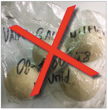
A sure indicator that a part has been pirated is its arrival in atypical packaging, such as valve balls that are delivered in simple plastic bags with the name and part number written in marker.
