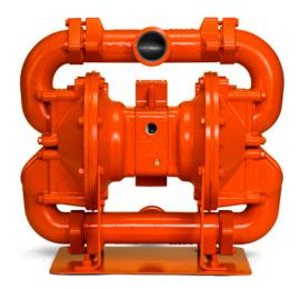
Wilden® Brahma® Series AODD Pumps have a unique top-inlet/bottom-outlet bolted design that allows them to effectively handle the passage of large solids with no risk of damage caused by product entrapment or the compromising of flow paths.
