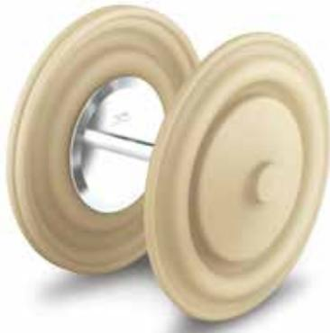
The Pure-Fuse Diaphragm has been designed with an integrated stainless-steel core that uses no adhesives or nylon fabric, which eliminates product-entrapment areas and greatly reduces contamination risks.
