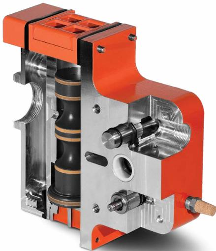
The Wilden® Pro-Flo® SHIFT ADS reduces air consumption while maintaining maximum operational efficiency and flow rates by restricting the air flow into the air chamber near the end of each pump stroke so that only the air required is introduced into the pumping process.
