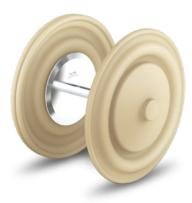
The new Chem-Fuse Integral Piston Diaphragm (IPD) from Wilden® reduces the risk that damaging product buildup will occur in AODD pumps through a design that encases the diaphragm's outer piston within the diaphragm material itself.
