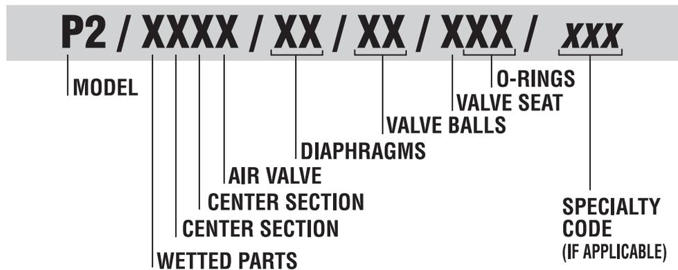
In the case where a center section is used instead of a center block and air chambers, the designation will be as follows: Polypropylene = PP
