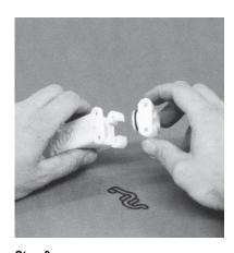
Remove air valve end cap by simply pulling it away from air valve body (no tools required). Inspect O-ring and replace as needed with genuine Wilden parts.
