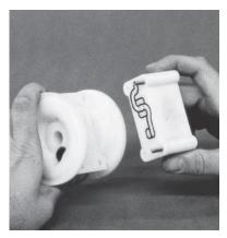
Take care while removing air valve not to damage gasket.
