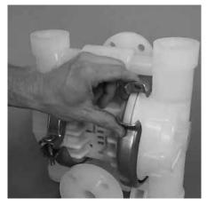
**Step 9**Rotate the clamp bands so that they can be removed.
