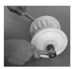
**Step 12**Using two 1" sockets, remove diaphragm assembly from center section assembly.
