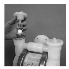
**Step 4**Remove the top liquid retainer to expose the valve balls, valve seats and valve seat o-rings.
