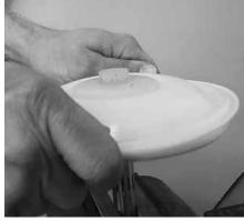
To remove the remaining diaphragm assembly from the shaft, secure shaft with soft jaws (a vise fitted with plywood or other suitable material) to ensure shaft is not nicked, scratched, or gouged. Using hands or an adjustable wrench, remove diaphragm assembly from shaft. Inspect all parts for wear and replace with genuine Wilden parts if necessary.
