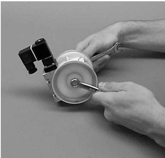
Step 10 Remove outer piston with 7/16" wrench if Rubber/TPE-fitted pump. For PTFE diaphragms, remove diaphragm by turning in a counter-clockwise direction.
