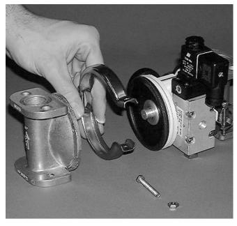
After clamp bands are removed, pull chambers away from center section.
