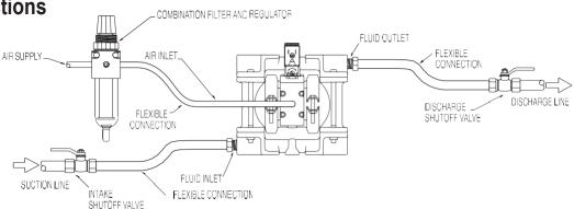
Accu-Flo™ pumps: Accu-Flo™ pumps function with solenoid valves and require an electrical control circuit to supply pulses. Under normal operating conditions, the control circuit is sufficient for starting and stopping the pump. However, the shut off valve (user supplied) installed in the air supply line can be used to stop the pump if necessary. Therefore, it should be located far enough away from the pumping equipment such that it can be reached safely in an emergency situation.
