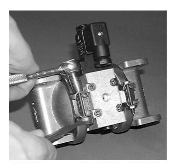
**Step 6**Loosen clamp band with 5/16" socket drive and 3/8" wrench. Remove screw and nut.
