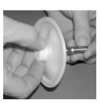
**Step 10**For PTFE fitted pumps diaphragms, remove diaphragm by turning in a counter-clockwise direction.
