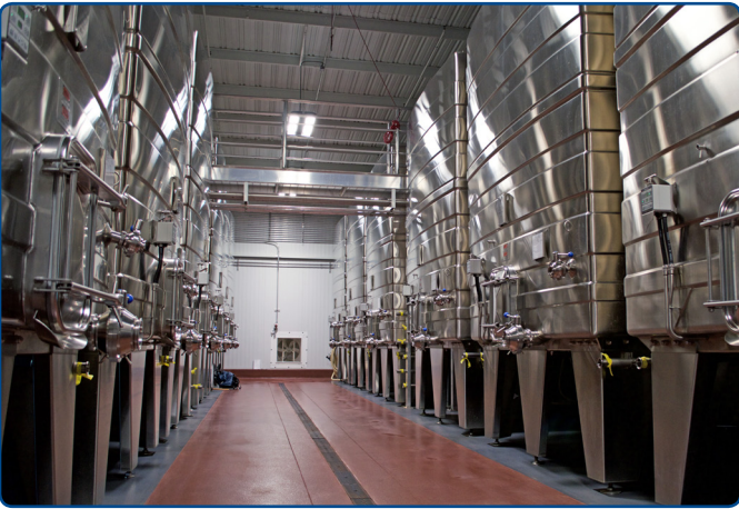
Rodney Strong's new 10,500-square-foot state-of-the-art cellar in Healdsburg, CA, USA utilizes 51 stainless steel 6,000-gallon fermentation tanks to accommodate premium grapes from their Cooley Ranch Vineyard.
