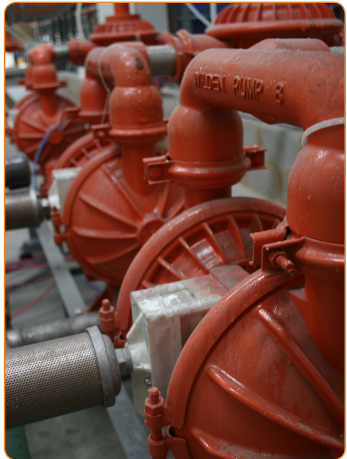
Because of their innovative design features, positive displacement AODD pumps often represent the best technology for handling “very searching” and aggressive liquids used during the manufacturing of high-performance coatings.
