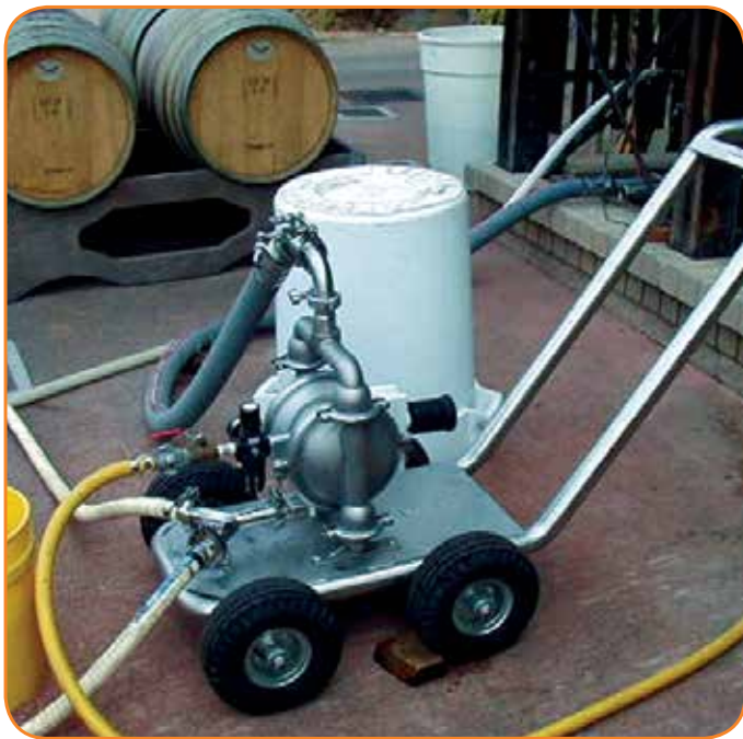
The operational advantages of using AODD pumps in winemaking processes are many, including easy to clean and maintain; gentle handling of delicate fluids; capable of moving large volumes; seal-less design; and portability.
