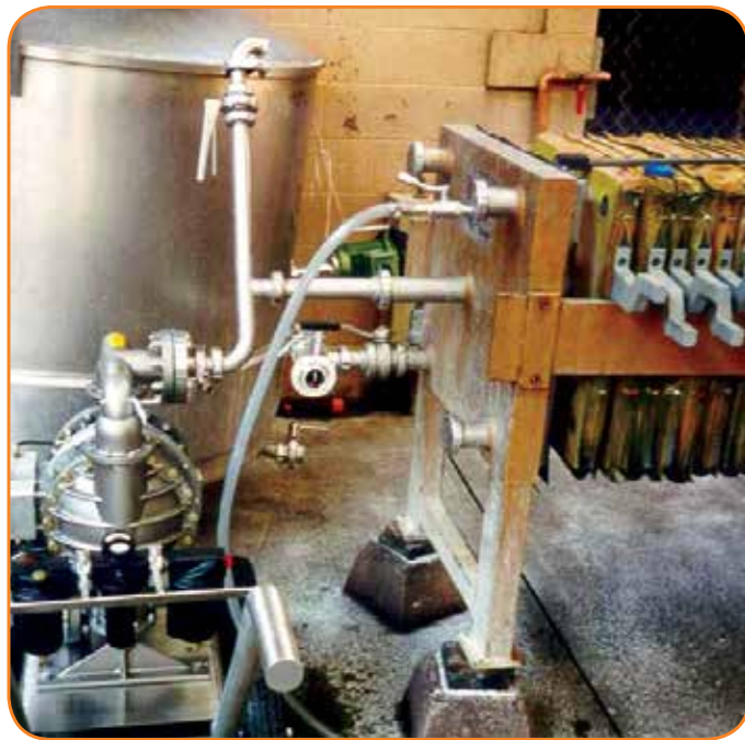
The operational advantages of using AODD pumps in winemaking processes are many, including easy to clean and maintain; gentle handling of delicate fluids; capable of moving large volumes; seal-less design; and portability.
