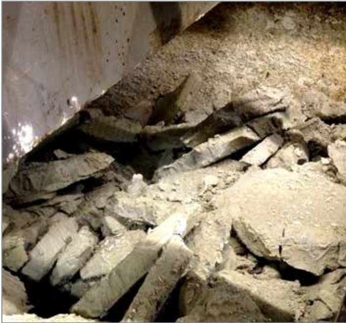
The facility's three filter presses process up to 9,600 gallons (36,340 liters) of waste sludge per day and produce more than 100 tons of "sludge cakes" per year.
