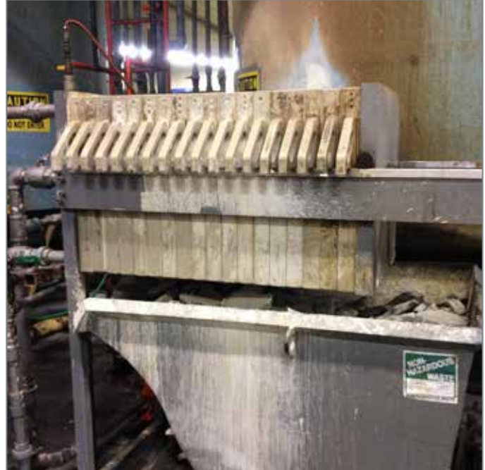
AMTROL's filter presses receive sludge containing water and metal particulate waste pumped by Wilden AODD pumps for separation into solid "sludge cakes" and water for safe, convenient disposal.
