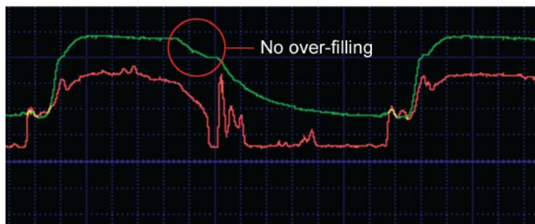
The chart above illustrates how the next-generation operation of the Pro-Flo® SHIFT ADS from Wilden® is able to eliminate the wasteful air overfilling that occurs at the end of each pump stroke with traditional AODD pump designs.
