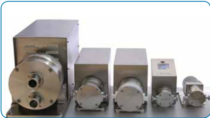
Quattroflow offers four sizes of quaternary diaphragm pumps to meet the needs of a wide range of biopharmaceutical manufacturing applications.
