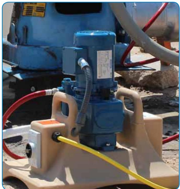
At the heart of this drip irrigation system is the Neptune 500-S Series metering pump.
