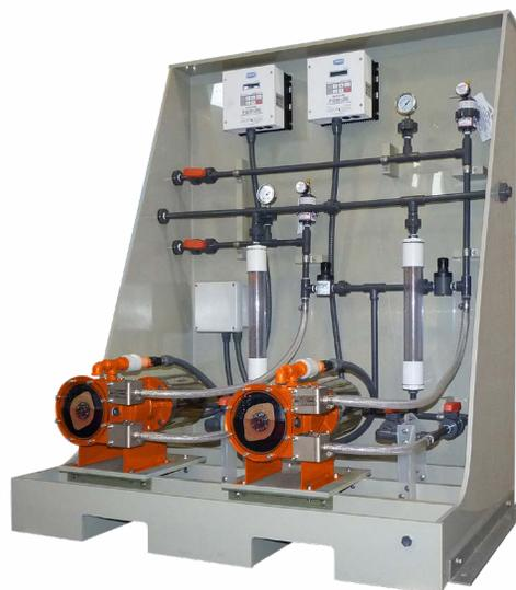
A wastewater-treatment plant's chemical-transfer system can be optimized through the use of peristaltic pumps because the technology does not contain any valves that can become clogged. This means that when the pump is shut down any viscous liquids that will generally solidify or become gelatinous when resting will not adversely affect the pump's operational capabilities.
