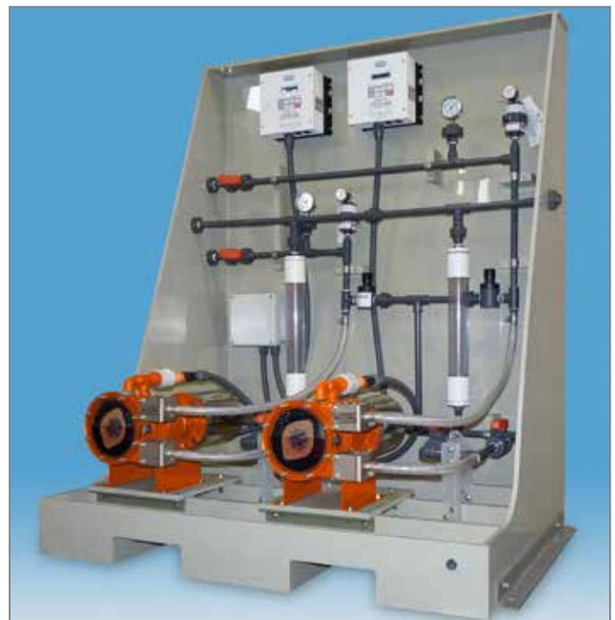
A wastewater-treatment plant's chemical-transfer system can be optimized through the use of peristaltic pumps because the technology does not contain any valves that can become clogged. This means that when the pump is shut down any viscous liquids that will generally solidify or become gelatinous when resting will not adversely affect the pump's operational capabilities.
