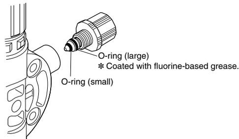
(3) Hold the retaining nut (the part shown by the arrow), turn it clockwise, and install it on the pump head.
