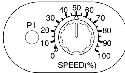
Adjustable range of stroke speed: 15 to 300 strokes/min
