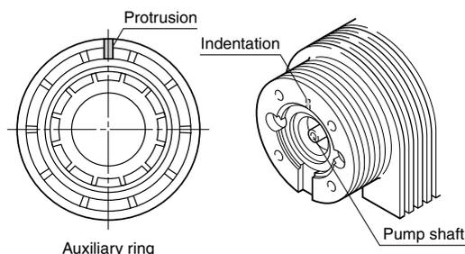
Align the indentation in the pump body with the protrusion of the auxiliary ring.
