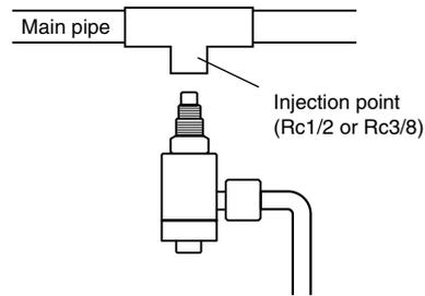
(2) Wind sealing tape around the external thread of the anti-siphon check valve, and screw the valve into the injection point.
