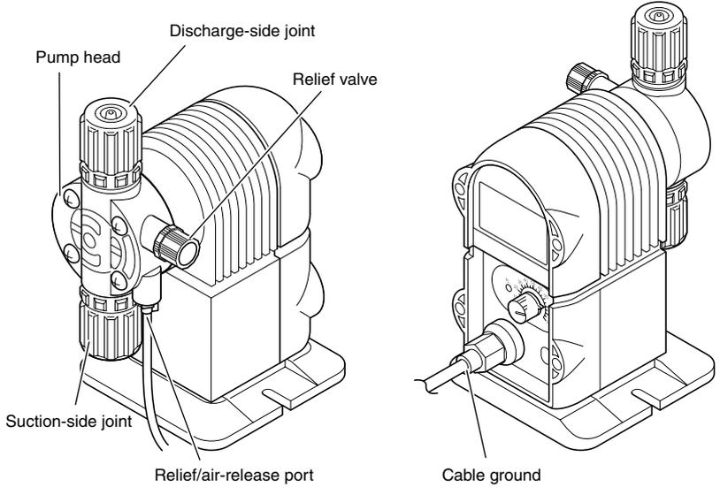
\* The shapes of pump heads and joints differ slightly depending on the liquid-end material and connection type.
