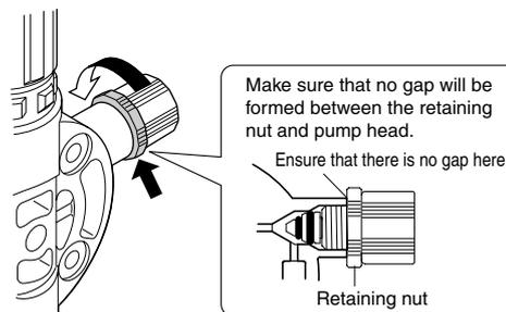
(4) After installing the relief valve, rotate the air-release knob by two turns in the clockwise direction to ensure that the O-ring is seated properly.
