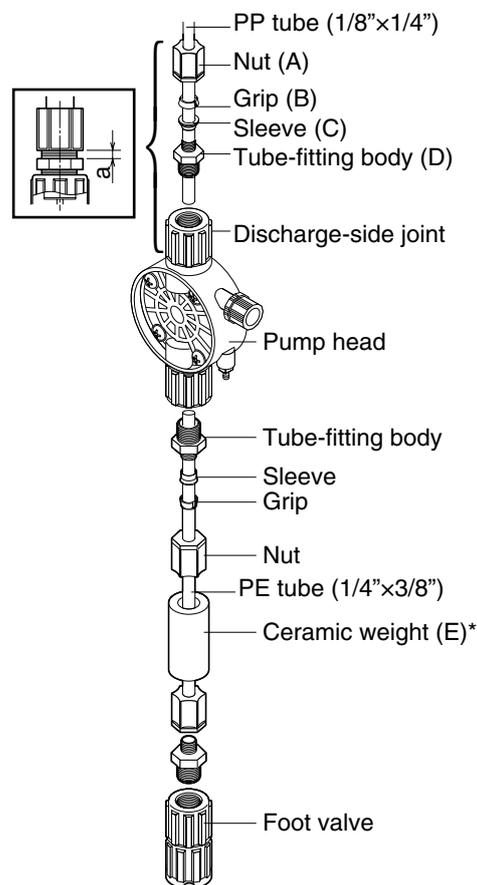
\* The tube is packed in the form of a coil. Attach the ceramic weight (E) and straighten out the tube so that the liquid inside the tank will be sucked up through it.
