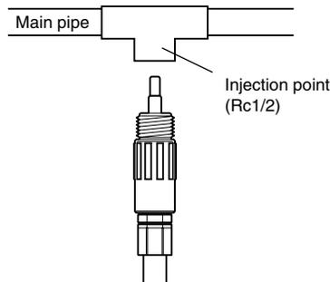
(2) Wind sealing tape around the external thread of the anti-siphon check valve, and screw the valve into the injection point.
