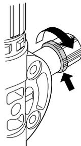
(2) Check the O-ring of the new relief valve for dirt or foreign matter.
