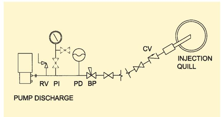
the maximum operating pressure. The relief valve return is piped back into the tank. Transparent return tubing allows fluid to be observed in the line if the relief valve opens. When portable, replaceable containers are used as the chemical source, it is convenient to pipe the relief valve back into the suction line. When piping the relief valve return to the suction, be certain the return is upstream of the pump suction isolation valve so that the flow path back to the tank cannot be blocked.
