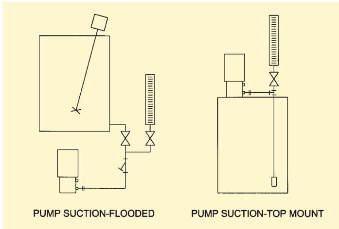
Flooded suction is always preferred in a metering-pump installation as it makes the pump easier to prime, but the length of the flooded suction should be limited to 6' or 7' (1.8 to 2.1 m). Flooded suction must be used for fluids where the vapor pressure could be less than the suction lift. And, as with all pump installations, adequately sized lines should be used and piping runs should have minimal bends, elbows or other design characteristics that may restrict or limit flow.
