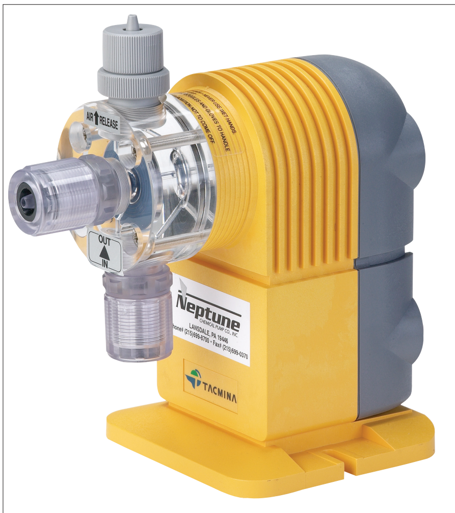
Figure 1: The key characteristic for the Series PZ electronic pump is its high stroking speed and short stroke length, making gas less likely to accumulate in the pump head.
