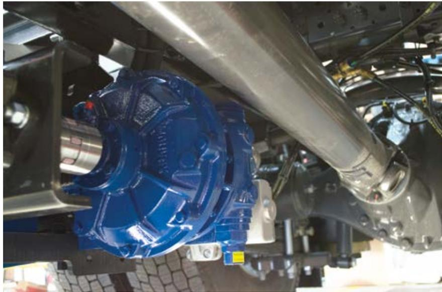
fluids that can be problematic for transfer pumps. The body and rotor of the Enterprise vane compressors are constructed of hard-coated cast iron that gives them the ability to withstand harsh operating conditions.
