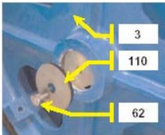
2. Remove the wheel **3** by sliding it on the shaft.
