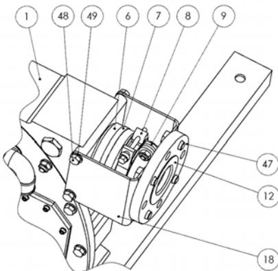
8. Mount flange **47** onto brackets **18** with the 2 screws **98** and 2 nuts **99** 180° apart.
