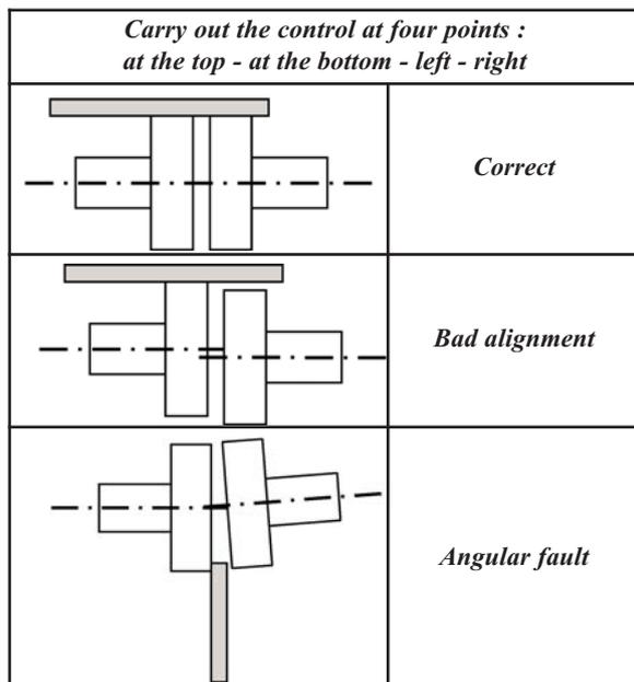
It is important to control the alignment at every step of installation in order to ensure that none of these steps generates stress on the pump unit or the pump itself :
