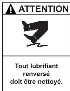
LE LUBRIFIANT DE LA POMPE EST TRES GLISSANT, ET PEUT OCCASIONNER DES BLESSURES GRAVES. IL EST IMPERATIF D'EN NETTOYER TOUT ECOULEMENT.
