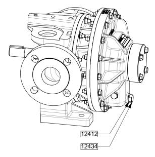
Once the pump is drained, fit the plug 12434 and its seal 12412.
