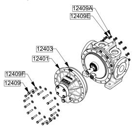
Remove the front cover bolts (screw 12409, nuts 12409A and washers 12409E - 12409F).
