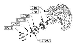
If necessary, fit the lip seal 12707, lip orientated outside in the bearing cover 12705.
