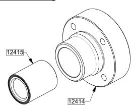
Orientate bushing chamfer on the outer side (see scheme above).
