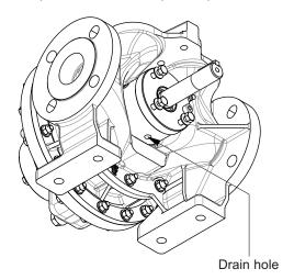
Fit the screws 12706 and theirs new ridged conic washers 12721 with medium thread lock.
