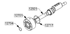
Remove the seal 12717 and check its condition. Replace it if necessary.
