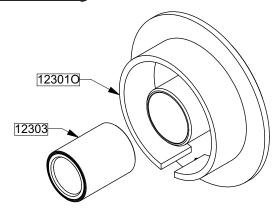
Insert the bushing 12303 in the piston 123010 with a press and a cylinder until the faces of the bushing and the piston are aligned (on both sides).
