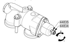
Setting is correct when flow rate is conform to expectation and when motor endures without incident absorbed power peak when discharge is closed. This is how relief valves of complete pumping sets are set, basing on information given to our technical services.
