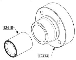
Remove the bushing 12415 of front cover bearing 12414 with a puller.
