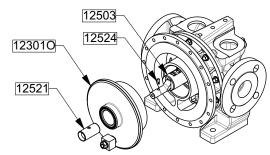
Lubricate the friction surfaces of the piston 123010 with a product compatible with the pumped liquid.
