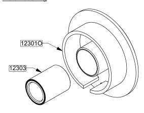
Remove the bushing 12303 of the piston 123010 with a press and a cylinder.
