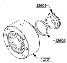
Remove the stationary seal face 12604 and its seal 12605.
