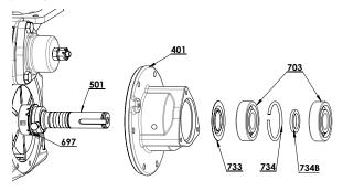
Once the end-plate is out, the rotating part 697 of the mechanical seal stays in place on the shaft. Caution not to scratch friction face.
