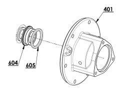
The introduction of the stationary seal face 604 and its seal 605 on the end-plate bore is done by hand up to stop. The rotating part of the mechanical seal 697 can be used to not scratch friction face. Otherwise use a clean, soft cloth.
