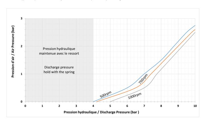
Check on the installation that the pump gives the right pressure (using a manometer) with a closed valve on the discharge line.
