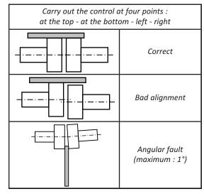
Controlling the alignment at each stage of the installation is important to be sure that none of the following procedures has generated stresses on the unit or the pump:
