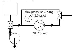
It is preferable not to run the SL Series pump during CIP although low speed (< 100 rpm) is acceptable by alternating start/stop operation.
