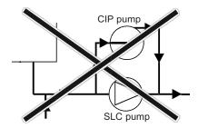
Indeed, in this case, the pressure at the inlet of the SL Series pump is lower than the pressure at the discharge and the piston remains forced against the cylinder. Therefore, there the SL Series pump no longer provides a passage. Its efficient cleaning can no longer be ensured and the cylinder/piston pair will become prematurely worn.
