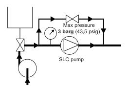
It is preferable not to run the SL Series pump during CIP, although low speed (< 100 rpm) is acceptable by alternating start/stop operation.
