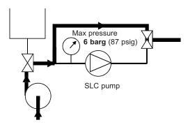
The pump must not run during this operation.
