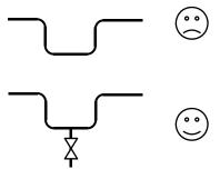
If installation is heated, it must be designed so that fluid dilatation can evacuate through piping. Therefore fluid contained in piping must be heated before fluid contained in the pump. Also check that a heated pump is not isolated by closed valves.
