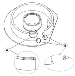
Before putting back the piston on the pump, eliminate these asperities by filing and finishing with fine sandpaper (No 320 grain or equivalent), taking care of not scratching any other surface around. Piston must then look as follows:
