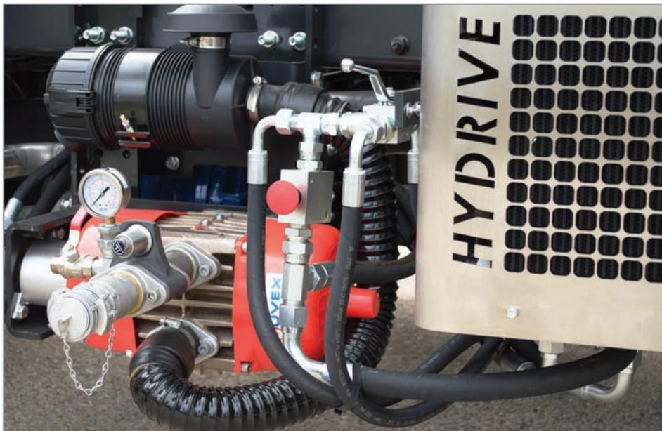
Mouvex® Enterprise Series Vane Compressors (left) and Hydrive® Hydraulic Coolers are ancillary equipment options that can be utilized when transport-truck loading and unloading activities need further optimization.
