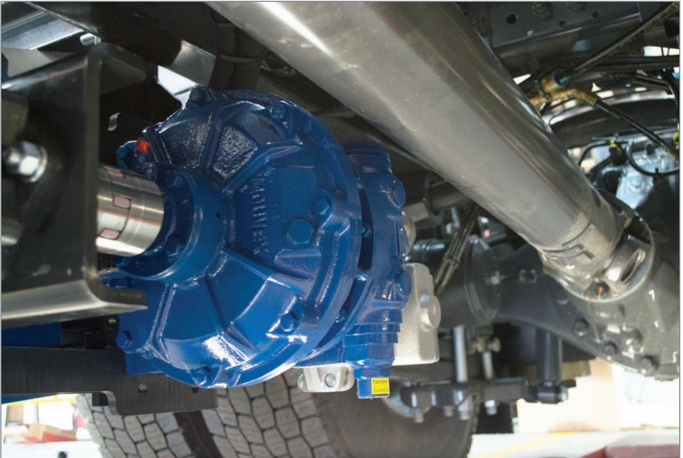
Mouvex® CC20 Series Eccentric Disc Pumps meet the needs of the European liquid and dry-bulk transport-truck market because their design and operation are perfect for the loading and unloading of a wide range of petroleum products, including gasoline, diesel, kerosene, heating oil, heavy oil, bitumen and biodiesel.
