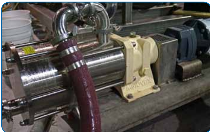
The Mouvex® C-Series eccentric disc pump helps Surly Brewing maintain consistency and quality by protecting yeast, proteins and malts against shearing.
