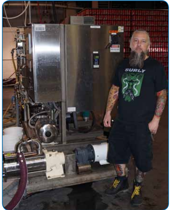
Head brewer Todd Haug (pictured) preferred the Mouvex® C-Series eccentric disc pump over commonly used rotary lobe pumps because it provided the minimum pulsation and gentle handling required when handling Surly's beer.
