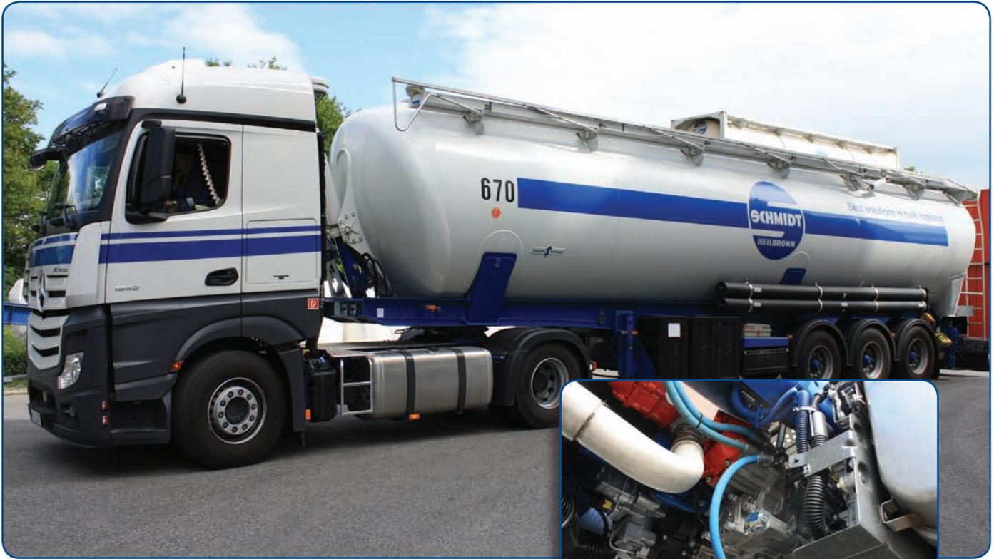
Responding to the stricter on-road diesel-emissions standards and weight requirements of the new Euro 6 regulation, as well as the safety and comfort needs of its drivers, The Schmidt Group has outfitted its dry-bulk truck fleet with MH6 Series Screw Compressors (inset) from Movex® and Hydrocar.
