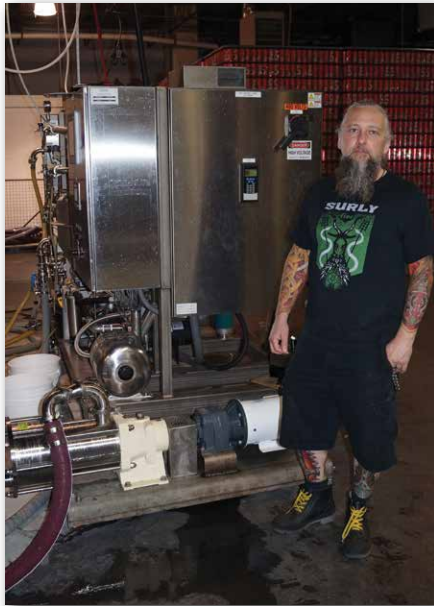
Head brewer Todd Haug (pictured) prefers the Mouvex® C-Series eccentric disc pump over commonly used rotary lobe pumps because it provides the minimum pulsation and gentle handling required for Surly's beer.
