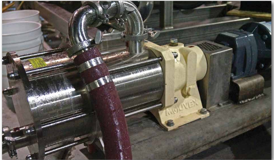
The Mouvex® C-Series eccentric disc pump helps Surly Brewing maintain consistency and quality by protecting yeast, proteins and malts against shearing.
