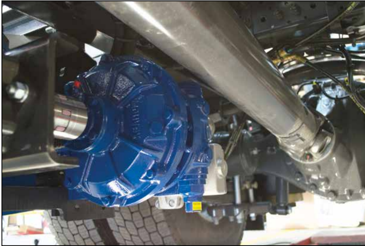
The CC20 Series Eccentric Disc Pumps meet the needs of the European liquid and dry bulk truck market because their design and operation are perfect for loading and unloading a wide range of petroleum products
