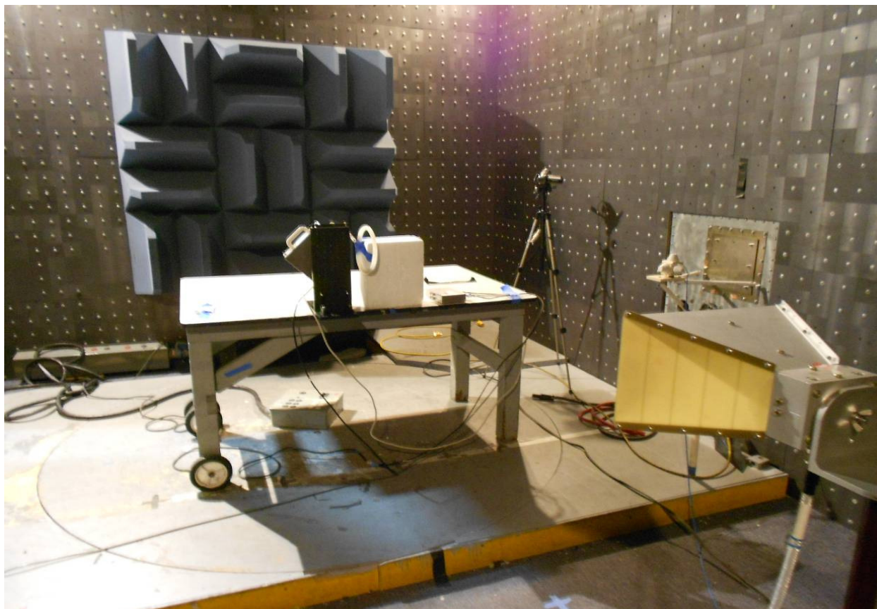
Test Configuration Photograph #2 (Radiated Immunity, EN 61000-4-3)
