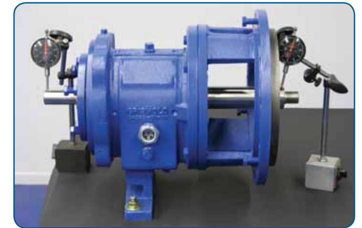
Shaft run-out must be checked at both the coupling end and the mechanical seal end. Maximum run-out is 0.002TIR.
