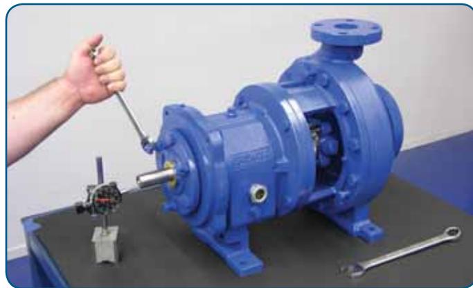
Impeller adjustment is made by turning the jack bolts at rear of bearing housing.
