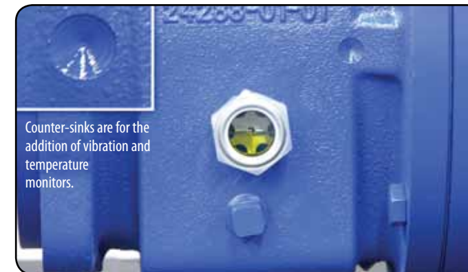
The oil level must be at the halfway point in the sight glass.
