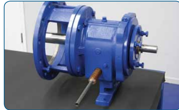
Temperatures above 350°F (117°C) require a finned tube oil cooler to cool the bearing frame.
