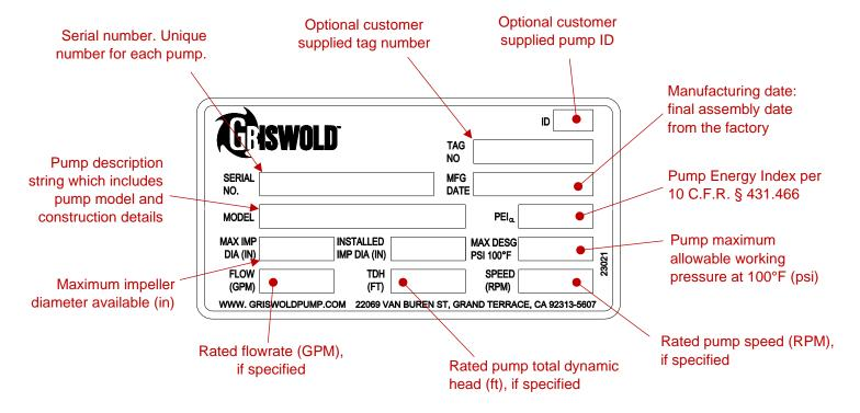
Each pump will be supplied with a factory installed nameplate. See the figure for a description of each nameplate field.
