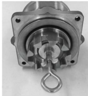
Rotor Assembly in Place
