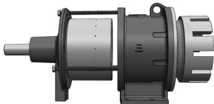
Separate Coupling with Jack Screws
