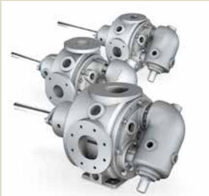
Image 2. Internal gear pumps feature a series of design enhancements that make them ideal for handling asphaltic products with a wide range of temperatures and viscosities. These include a large jacketed surface on the pump case and pressure relief valve, jacketing behind the pump rotor, a rotatable casing and high-strength, ductile-iron gear material.
