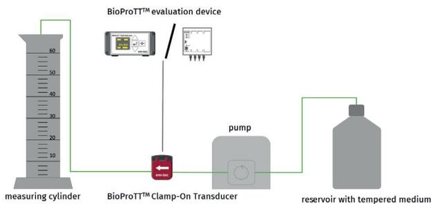
Figure 5: Setup Volume Over Time
