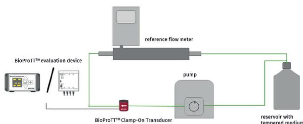
Figure 3: Setup Coriolis
