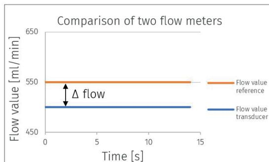
Figure 4: Comparison of Two Flow Meters
