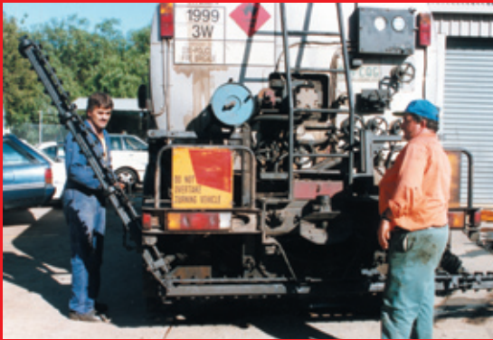
Road Sprayer equipped with EBSRAY G Series Pump & EBSRAY SB Series Spraybar
