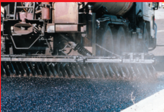
Road Sprayer in action - note even distribution from G Series pump.
