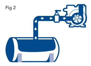
This illustration shows how wetted suction lift works. With the sliding vane pump positioned above the liquid source and with residual liquid inside the pump (Fig 1), the liquid is drawn up and into the pump, creating a wetted condition (Fig 2).
