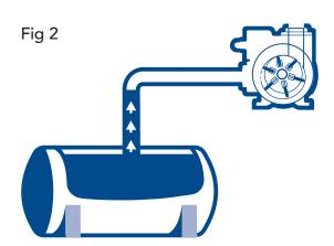
This illustration shows how the concept of dry suction works. With the sliding vane pump located above the liquid source (Fig 1), the pump's "self-priming" capability allows it to create a vacuum that can pull the liquid up toward the pump chamber (Fig 2).
