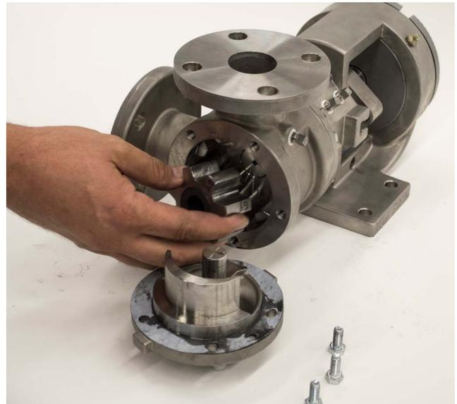
*G Series Internal Gear Pumps feature a unique design that features only two moving parts, a rotor and idler gear, which allows them to operate equally well in either direction and deliver positive, non-pulsating flow of the liquid being handled.*
