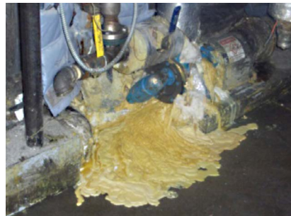
These are a few examples of what can go wrong when pump styles with inadequate product-sealing capabilities are used in resin-handling applications.
