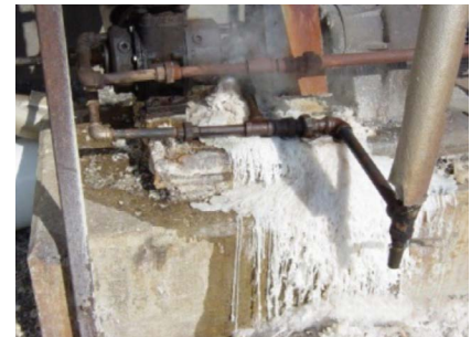
These are a few examples of what can go wrong when pump styles with inadequate product-sealing capabilities are used in resin-handling applications.
