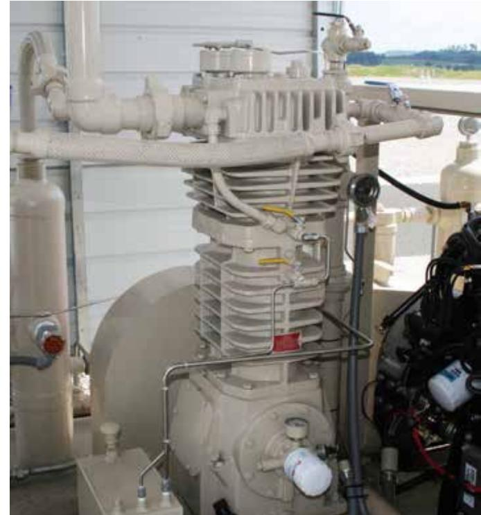
*Blackmer® offers its HD (shown), HDS and NG Series models of Reciprocating Gas Compressors for use in oilfield applications.*
