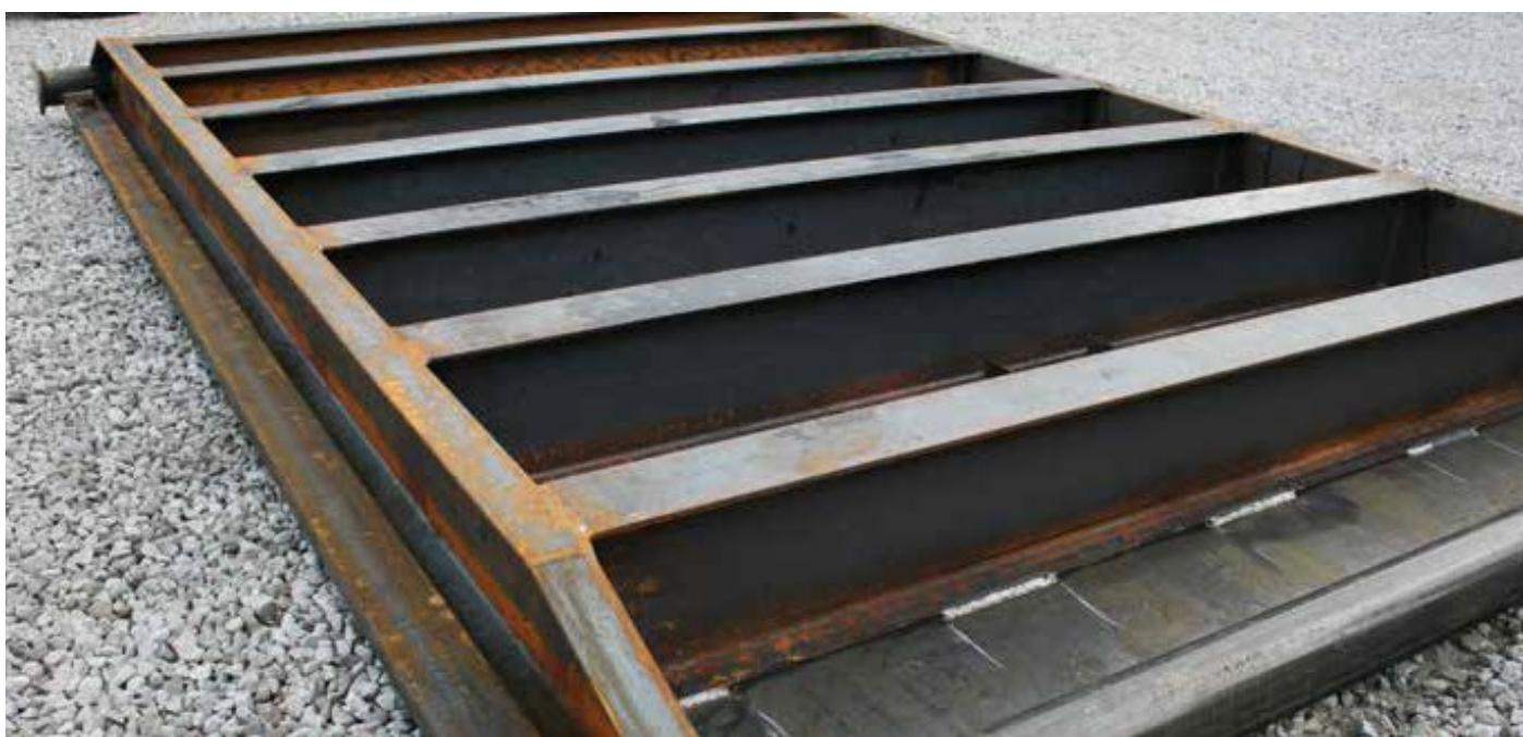
*A key to effective vapor-recovery unit operation in the oilfield is the skid on which it rests. This skid assembly must be the proper weight and anchored correctly if it is to effectively absorb the shaking forces and moments that are produced by the VRU's compressor.*
