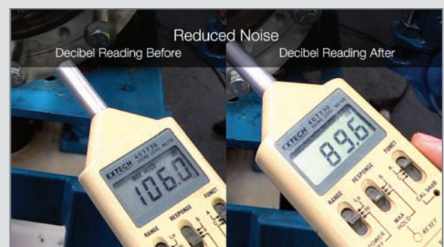
The pump operating without a Cavitation Suppression Liner produced a noise level of 106 decibels (left) compared to 89.6 decibels for the pump with a Cavitation Suppression Liner.
