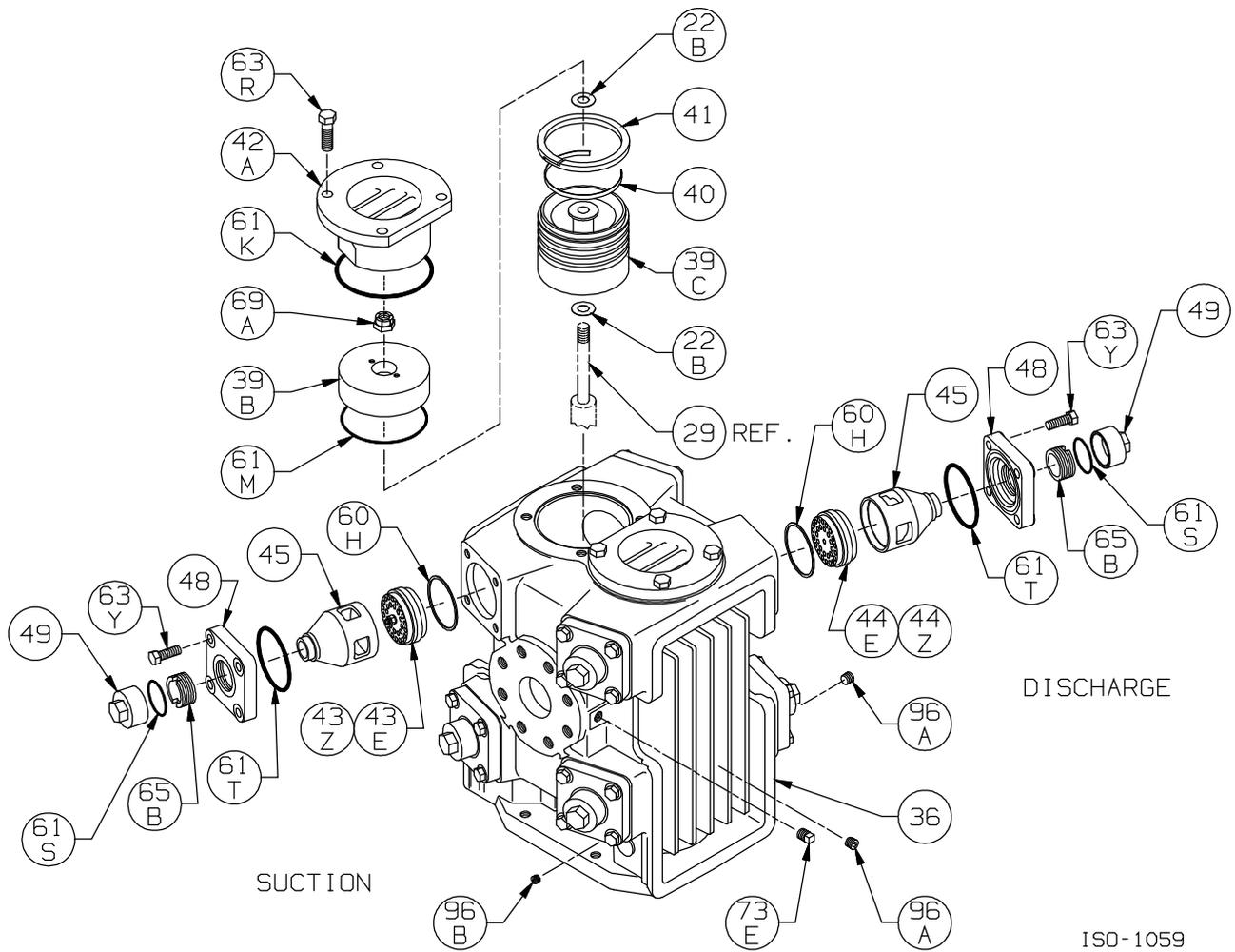
Cylinder Assembly: HD942B, HD942A, HD943B
