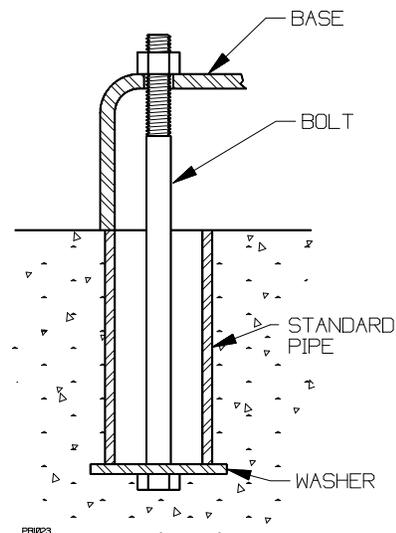
**Figure 2 - Anchor Bolt**
