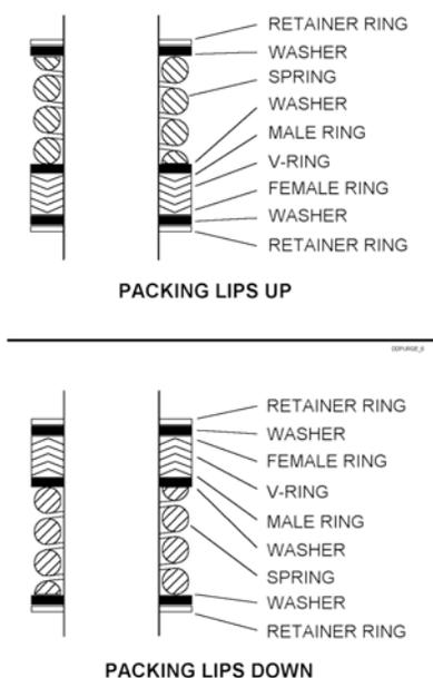
**Fig. 11 – Seal Component Orientation**
