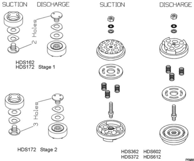
**Fig. 10 – Typical Valve Assemblies**
