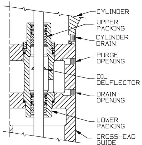
Fig. 3 - TYPICAL SEAL AREA CONSTRUCTION
