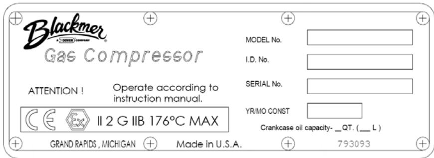
**Figure 2 - Compressor Nameplate**
