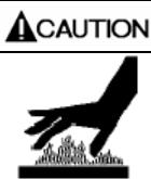
**Discharge piping surface temperatures may be hot during operation (over 158°F, 70°). Temperatures should be monitored and adequate warnings posted.**
