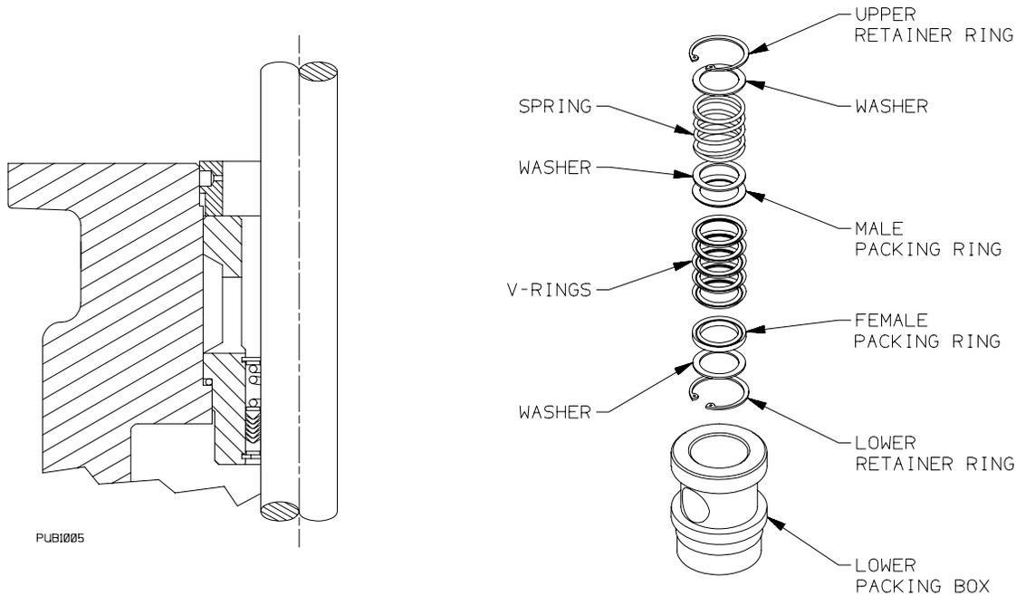
Figure 20 - Lower Packing Assembly
