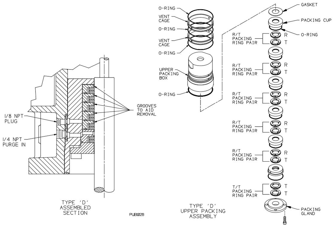
Figure 19 - Type 'D' Packing Detail
