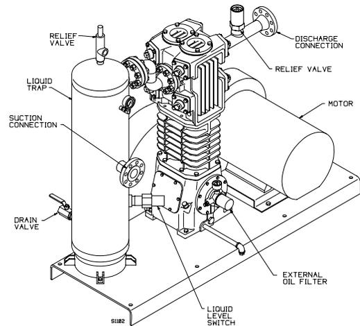
**Figure 5 – Typical HD942 Compressor Package**
