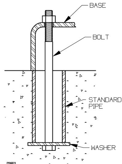
**Figure 3 - Anchor Bolt**
