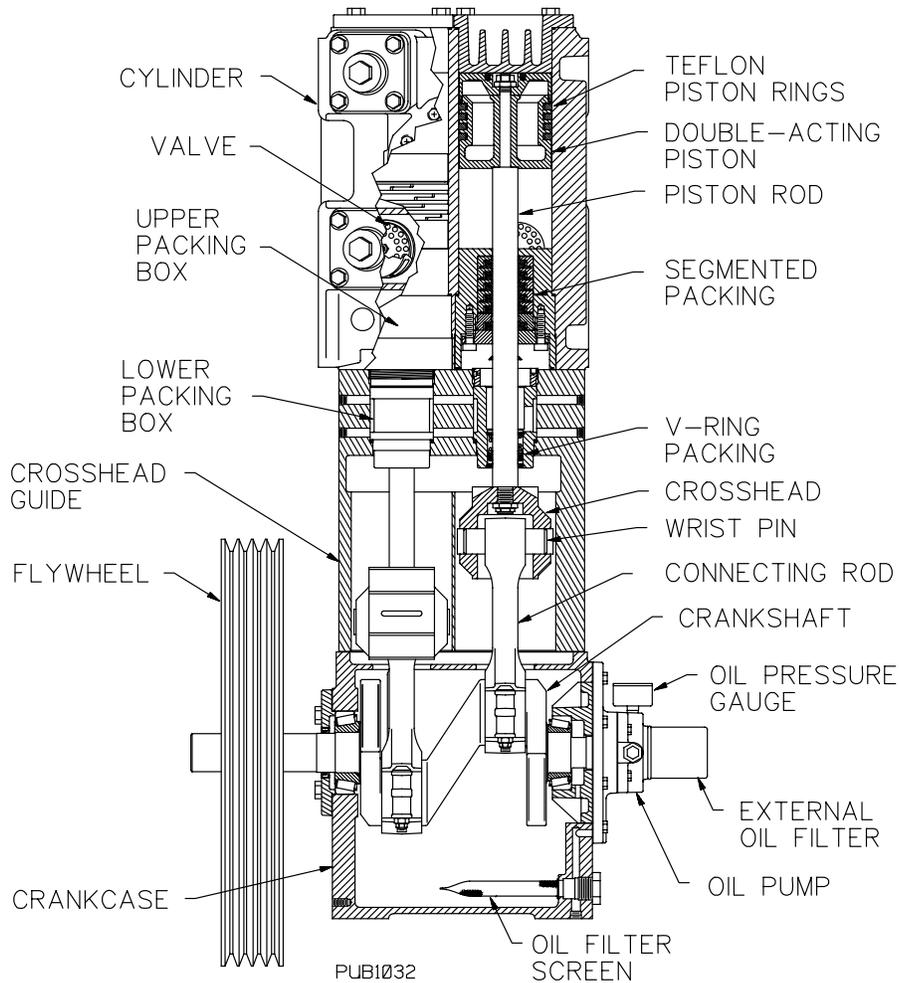
**Figure 1 – Air-Cooled HD942A Compressor (Type 'B' Packing shown)**
