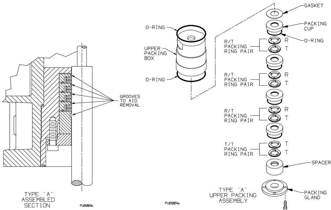
**Figure 16 - Type 'A' Packing Detail**
