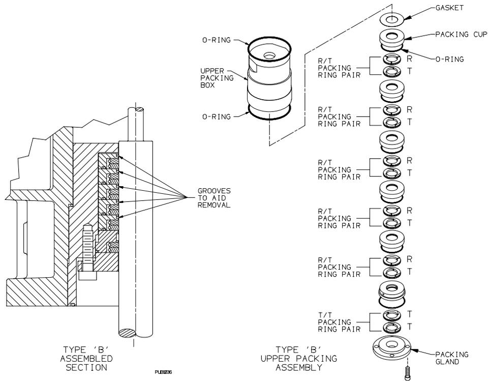
Figure 17 - Type 'B' Packing Detail
