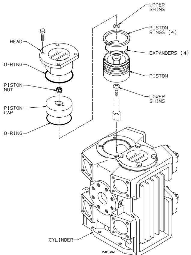
Figure 7 - Cylinder and Piston
