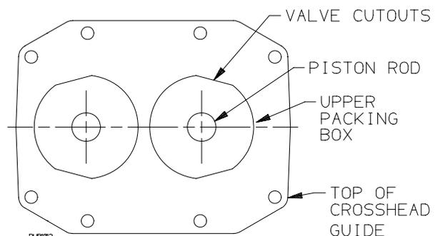
**Figure 9 - Upper Packing Box Alignment**
