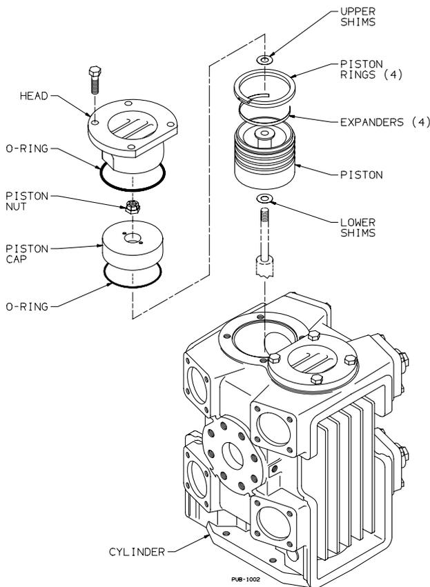
**Figure 10 - Cylinder and Piston**
