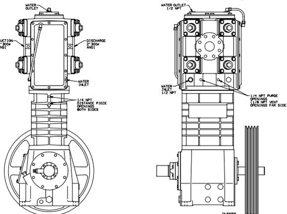
Figure 4 - HDL942 Water Connections
