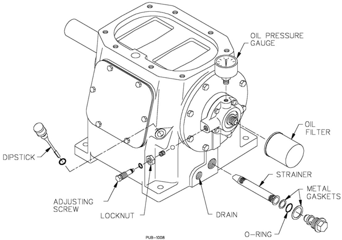
**Figure 6 - Compressor Lubrication System**
