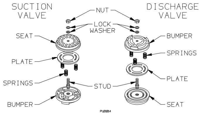
Figure 13 – Ductile Iron / PEEK Valve Detail
